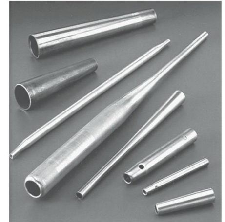
(a) Schematic illustration of the rotary-swaging process. (b) Forming internal profiles on a tubular workpiece by swaging. (c) A die-closing swaging machine, showing forming of a stepped shaft. (d) Typical parts made by swaging..
